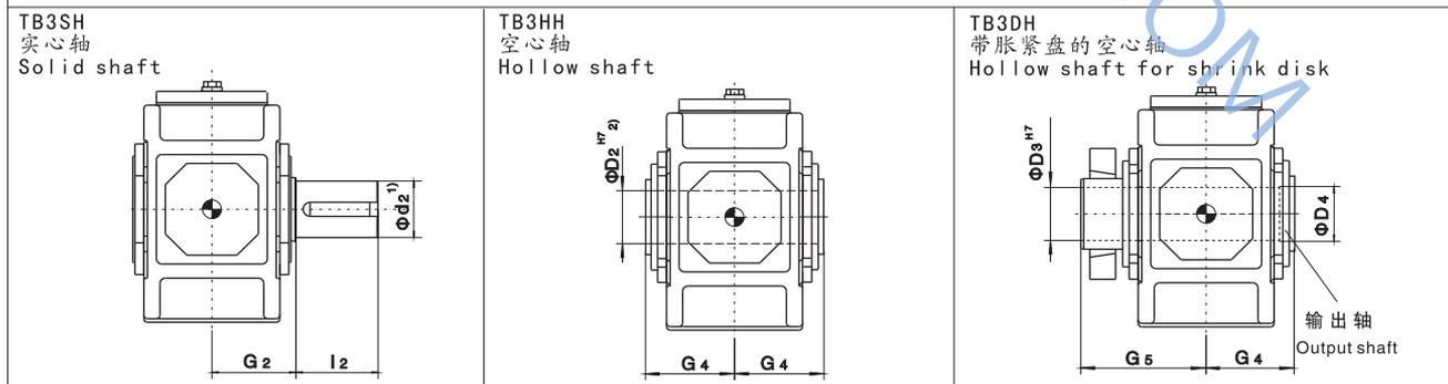
1)  $k6 \leq \Phi 25$   $\Phi 28 \leq m6 \leq \Phi 100$   $n6 > \Phi 100$       1)  $k6 \leq \Phi 25$   $\Phi 28 \leq m6 \leq \Phi 100$   $n6 > \Phi 100$
